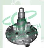
Delivery Ports: (4) 1/4" NPT Supply Ports: (1) 1/4" NPT Control Ports: (1) 1/4" NPT Reservoir Ports: (1) 1/2" NPT Normal Crack Pressure: 1.5 PSI Replaces: Sealco A1000S
